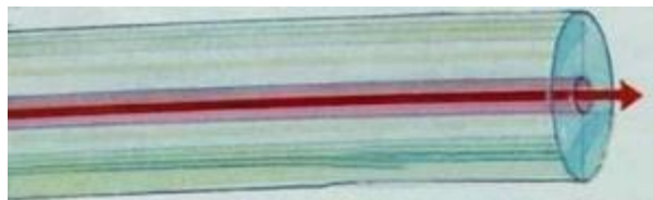
Gambar 3.2. Jenis Fiber Optik Single mode fiber
